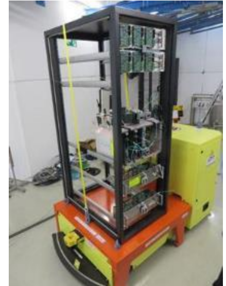
CHARM mixed-field facility: GeV proton beam on copper target; tailored to test multiple boards or full systems
