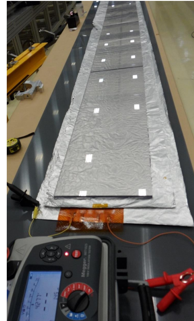
Quench heater high voltage test of (a) series heater and (b) heater encapsulated with polyimide coverlay.
