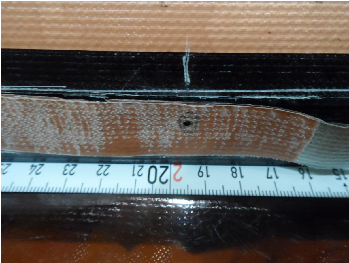
Peeled off metallic circuit
