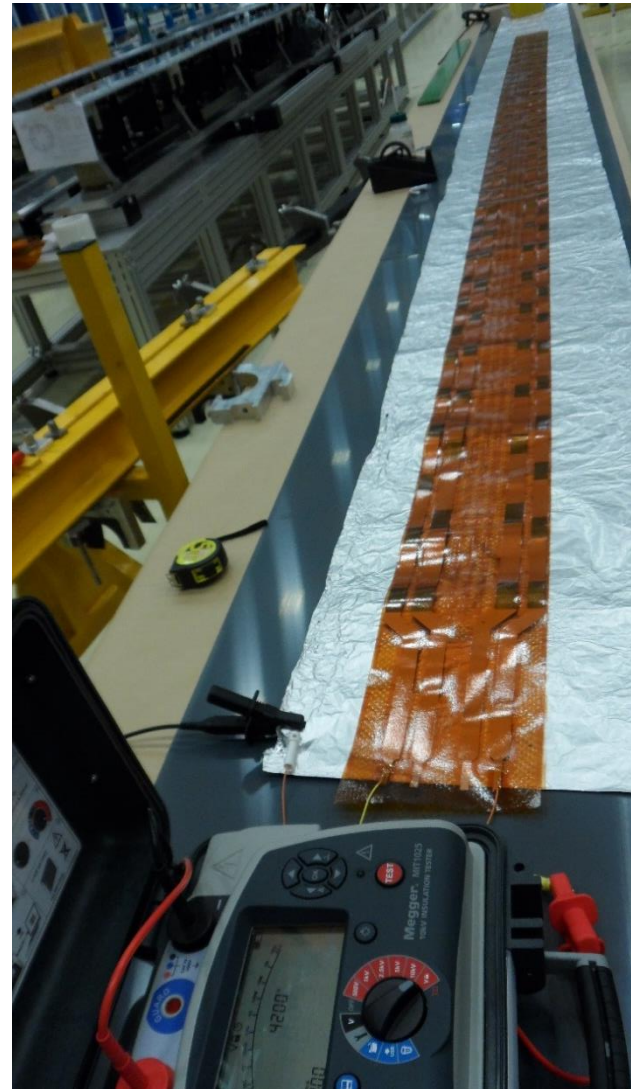
Quench heater high voltage test of (a) series heater and (b) heater encapsulated with polyimide coverlay.
