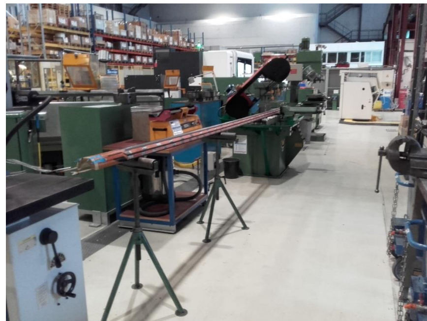
Rough cutting of coil CR06.
