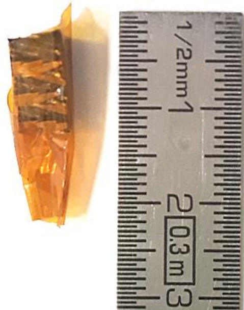
Sample with defect for \mu -CT examination
