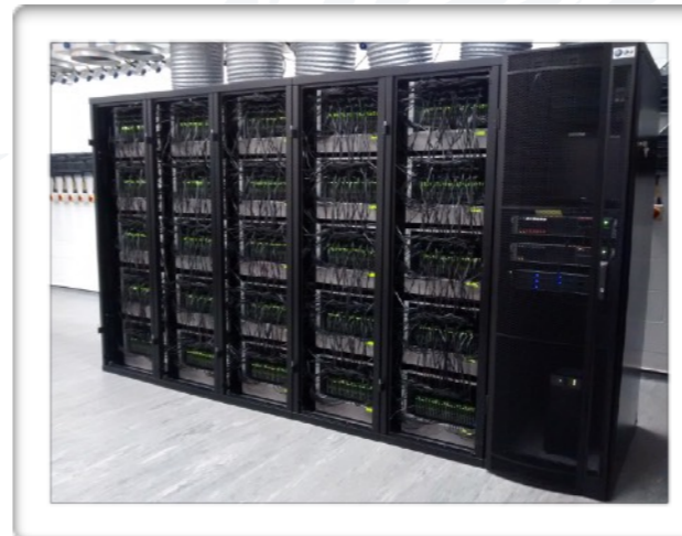
2016: Spinnaker 0.5M core machine @ HBP/Manchester
