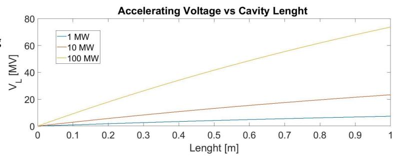
Average accelerating voltage vs incident power for different structure lengths
