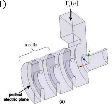
D. Alesini et al., Design of couplers for traveling wave RF structures using 3D electromagnetic codes in the frequency domain, NIM-A (2007)
