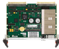
VME Card: Eurocard size VMEbus interface
