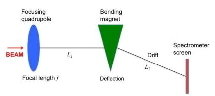
1. If the effective length of the dipole is  $l_B = 0.43$  m, what should be the magnetic field (in Tesla) inside the dipole to deflect the electrons by an angle of 35 degrees?
