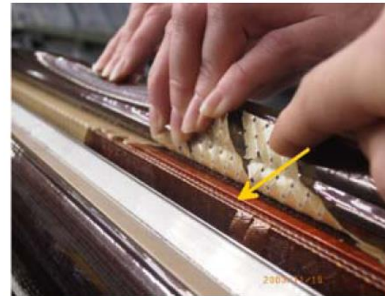
Fig. 9. Left: Movement of block 6 of the inner layer of the coil observed after de-collaring. Right: Illustration of the predicted defect and block numbering.
