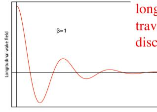
Causality requires that the longitudinal wake field of a charge travelling with the speed of light is discontinuous in the origin.
