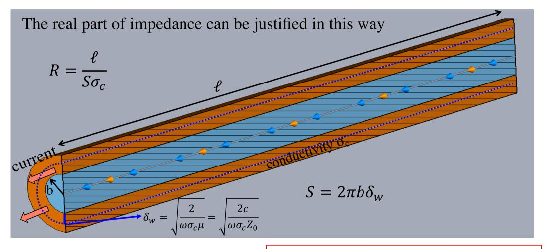
$$R = \frac{\ell}{2\pi b \delta_w \sigma_c} = \frac{\ell}{2\pi b} \sqrt{\frac{Z_0 \omega}{2c\sigma_c}} \quad Z_{//}(\omega) = [1 - i \operatorname{sgn}(\omega)] \frac{\ell}{2\pi b} \sqrt{\frac{Z_0 |\omega|}{2c\sigma_c}}$$
