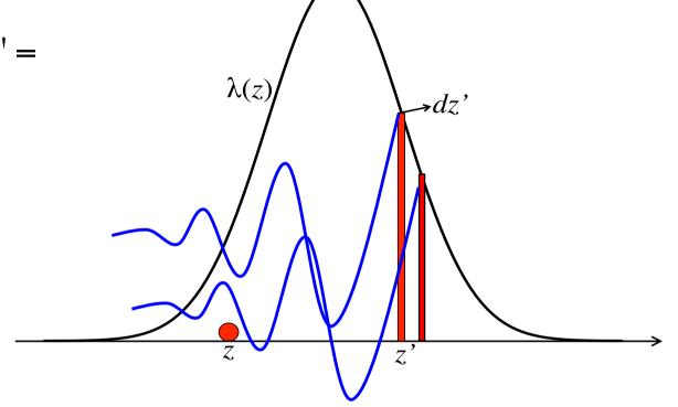
The energy lost allows to define the *longitudinal wake potential of a distribution*
