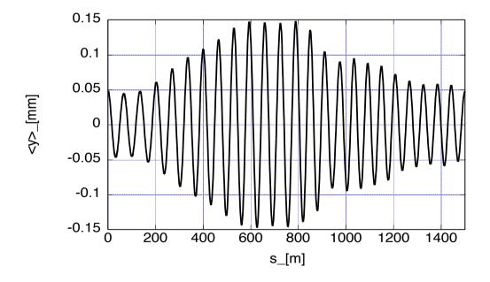
by a suitable choice of  $\Delta \omega_y$ , it is possible to fully depress the oscillations of the tail.
