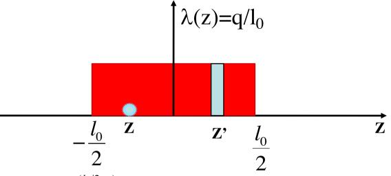
$$U(z) = -\frac{eqw_0}{l_0} \int_0^{(l_0/2-z)} \cos\left(\frac{\omega_r}{c}x\right) dx = -\frac{eqw_0}{l_0} \left[ \frac{\sin\left(\frac{\omega_r}{c}x\right)}{\left(\frac{\omega_r}{c}\right)} \right]_0^{(l_0/2-z)}$$
