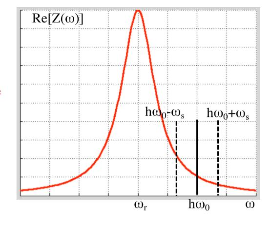
$$\alpha_r = \frac{eN_p \eta h \omega_0}{\omega_s (E_0 / q) T_0^2} \text{Re}[\Delta Z]$$
