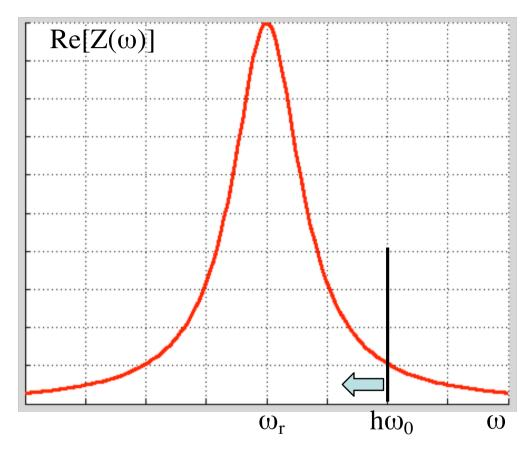
If  $(h\omega_0 > \omega_r)$ , as in the figure, the resistance found by the beam is higher, producing a higer energy loss, which reduces the energy increase giving a stabilizing effect.
