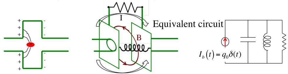
Each mode can be treated as an electric RLC circuit loaded by an impulsive current. Just after the charge passage, the capacitor is charged with a voltage  $V_o = q_o / C$  and the electric field is  $E_{so} = V_o / l_o$ .
