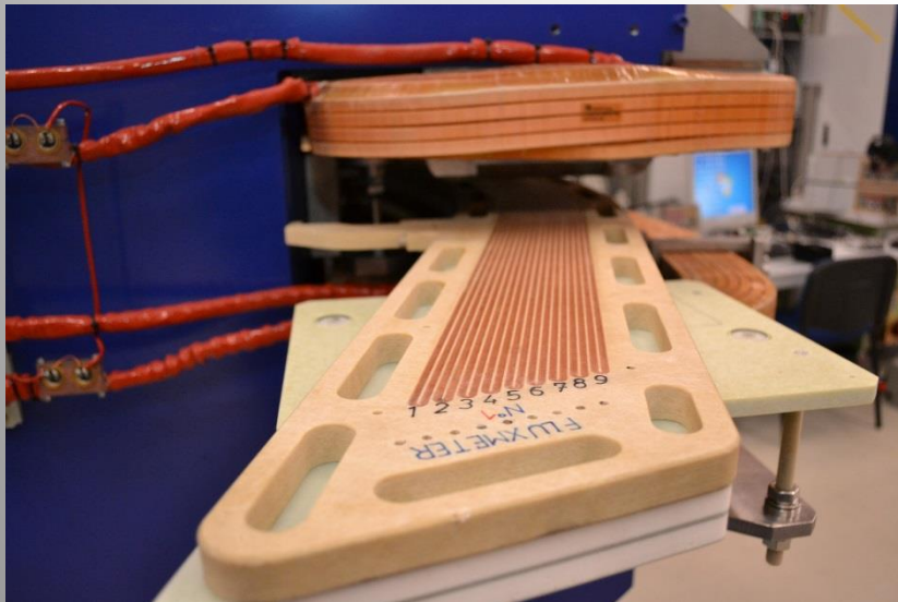
Nine-coil fluxmeter for the ELENA B-Train
