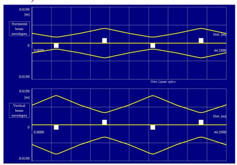
Inverter with skew quads powered.
