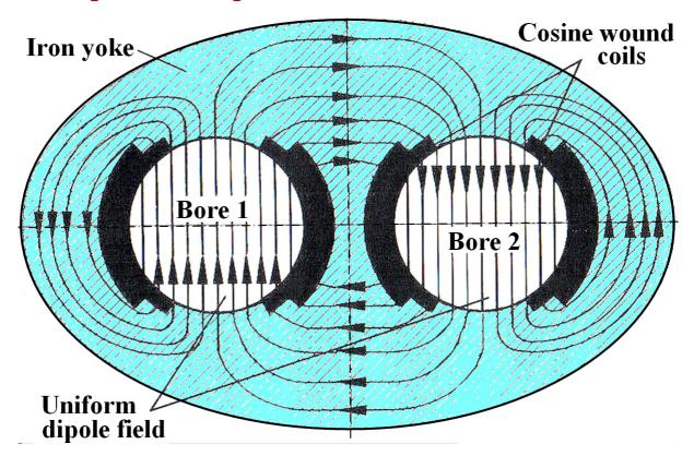
**❖** The twin-bore design is used in the LHC. This choice was driven mainly by the lack of space in the already existing LEP tunnel.
