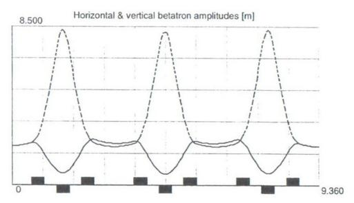
**The sigma matrices can be used to track the beam sizes through the rotator.** Terms  $m_{11}$  and  $m_{33}$  give the beam width and height on the orthogonal p-q planes (see last lecture).
