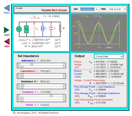
Change in the plot field (upper right corner) the setting from 'Voltage and current' to 'Resonance'
