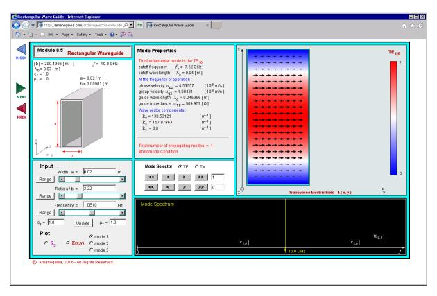
With help of page 16 "Mode chart of a rectangular waveguide" of the JUAS RF Course 2016 you can visualize the field pattern of the different modes in the transverse plane.
