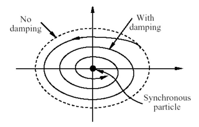
The derivative  $\frac{dU_0}{dE}$  (>0) is responsible for the damping of the longitudinal oscillations
