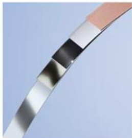
Fig. 1. A 12 mm tape produced by BHTS via ABAD and PLD method.
