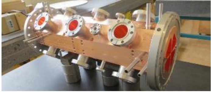
Radio Frequency Quadrupole linac system for isotope production in hospitals (CERN)
