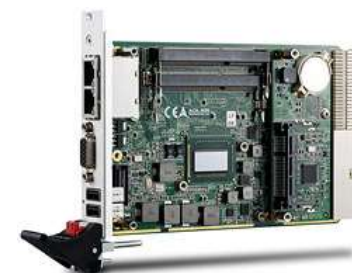
cPCI & Intel i7 + ADC-DAC for LLRF, BPMs
