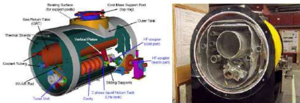
Figure 6-1: Cut-away diagram of an XFEL vacuum vessel.
