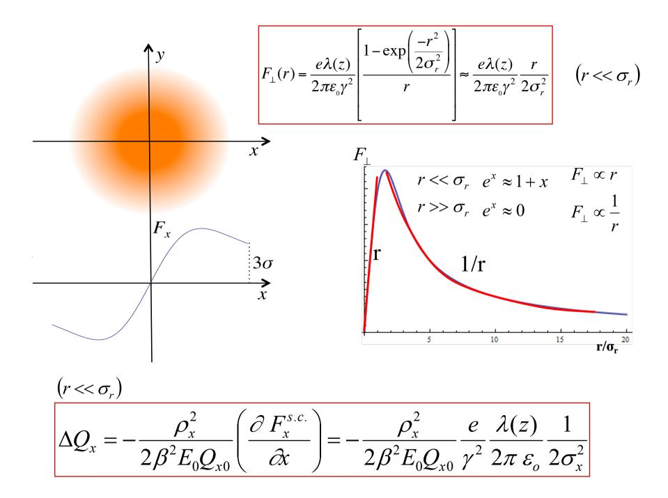
If the charge distribution is Gaussian but with different  $\sigma_x$  and  $\sigma_y$  (not cylindrical geometry), it is still possible to obtain the transverse electric field. The expression is known as Bassetti-Erskine formula: M. Bassetti and G.A. Erskine, "Closed expression for the electrical field of a two-dimensional Gaussian charge", CERN-ISR-TH/80-06 (1980).
