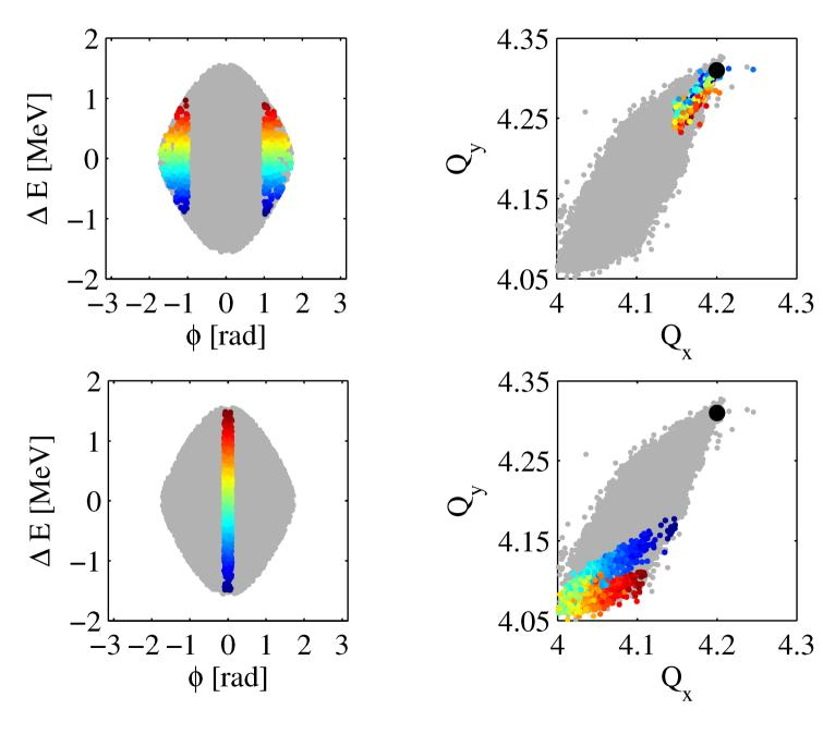
Longitudinal phase-space  $(\Delta \phi, \Delta E)$  scatter plot of the bunch tune footprint. The black dot is the bare tune. Particles at the edges of the bunch have tunes close to the bare tune in the necktie.
