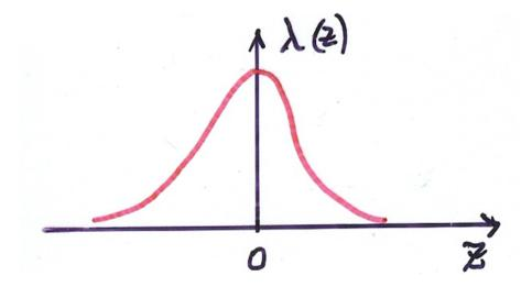
$$\Delta Q_{\max} (\text{at } z = 0) = -\frac{\rho_x^2 r_{e,p}}{\beta^2 \gamma^3 a^2 Q_{x0}} \frac{N}{\sqrt{2\pi}\sigma_z}$$
