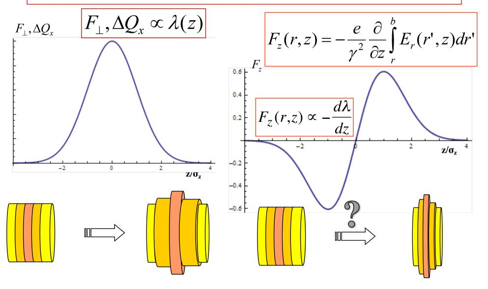
Compute the longitudinal space charge force of a transverse uniform cylindrical beam in a circular perfectly conducting beam pipe
