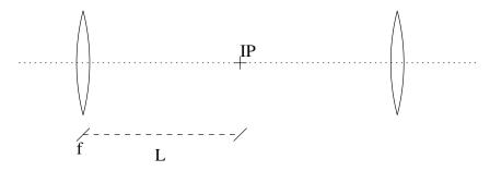
The beam enters the quadrupole with Twiss parameters  $\beta_0 = 20$  m and  $\alpha_0 = 0$ . The drift space has length L = 10 m.
