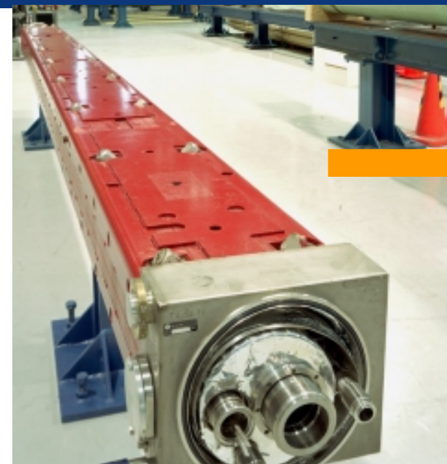
Tevatron dipoles: 4.2 T single aperture, warm yoke
