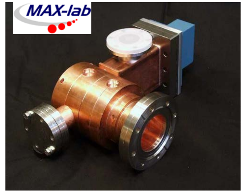
A 3 GHz thermionic RF gun has been designed. It will produce a 2.3 MeV electron beam with bunch charge up to 0.2 nC (600 mA) at 10 pmm mRad normalised emittance.
