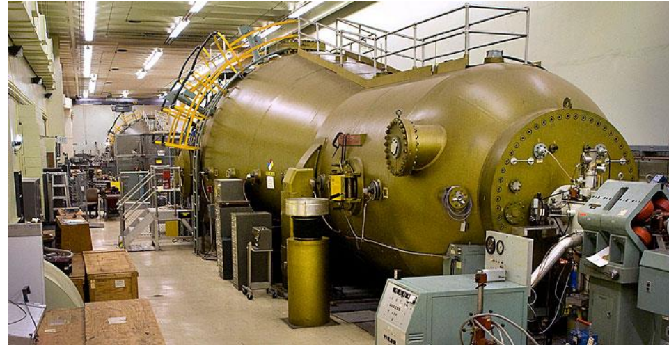
2 x 15 MV tandem Van de Graaf at BNL To raise electrical breakdown limits, the machine is contained in a SF 6 tank under pressure
