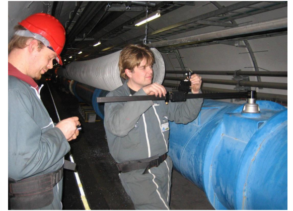
Manual device Accuracy 0.07mm
