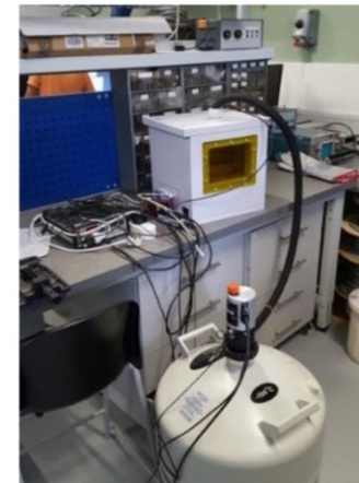
Cold box in the lab in Sheffield, ready for installation in Birmingham's cyclotron. (Image: Richard French)
