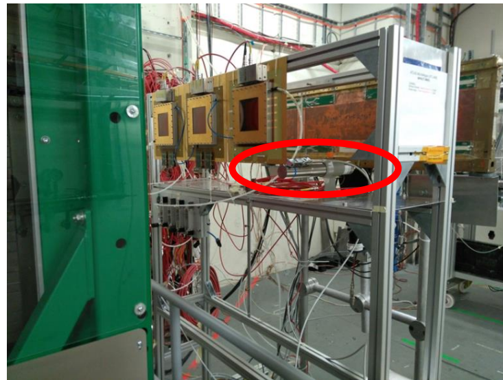
position of the RADMON+ Berthold GM Upstream and Downstream at Gif++
