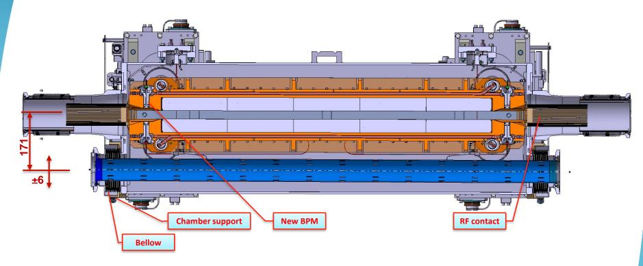
The position of the chamber of the 2<sup>nd</sup> beam can be adjusted to use the same tank for TCLPX and TCTPXH
