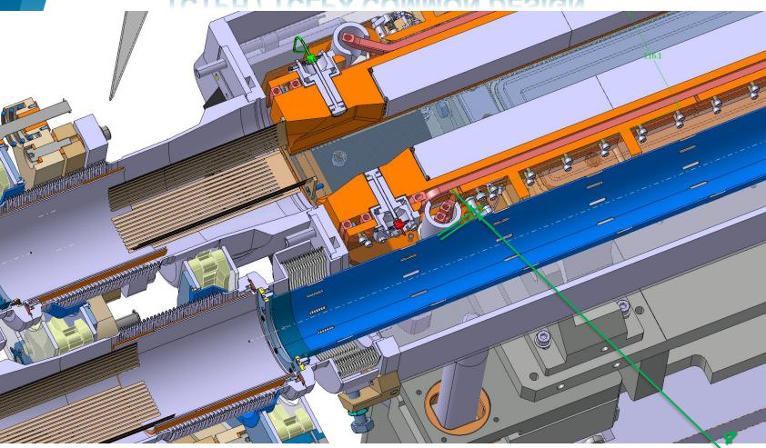
Very limited space between the TCLPX jaw and 2<sup>nd</sup> beam chamber. To reduce stroke and chamber dimension the remote alignment is very beneficial .
