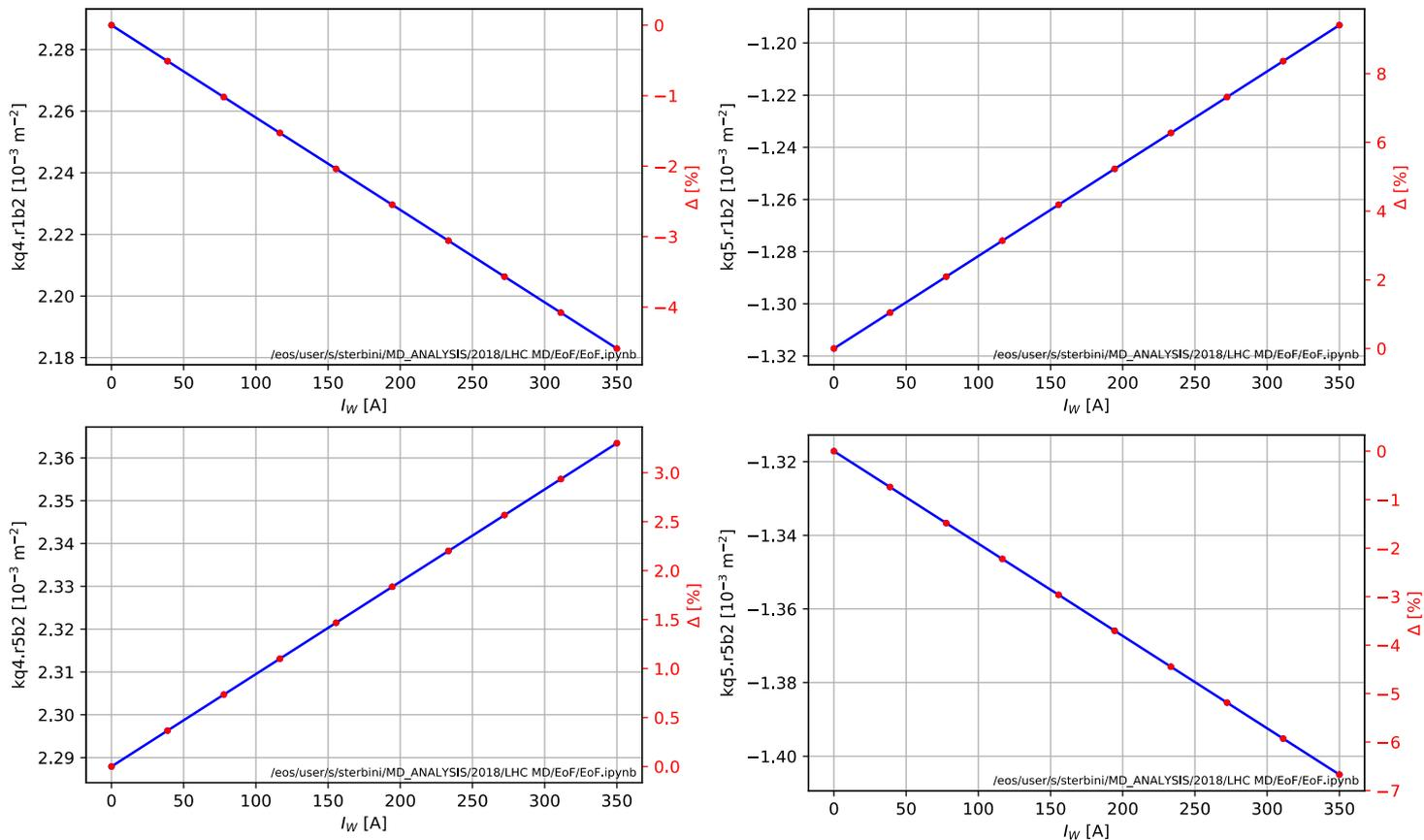
When we trim a wire the Q4/5 close to the wire are trimmed to compensate as close as possible the quadrupolar perturbation of the wire.
