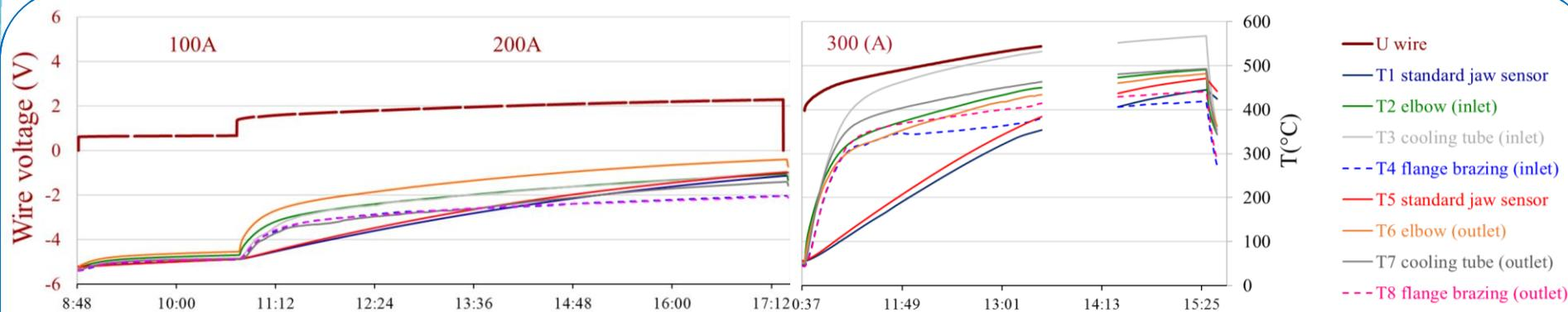
Tests performed on spare wire-in-jaw, under vacuum with no coolant
