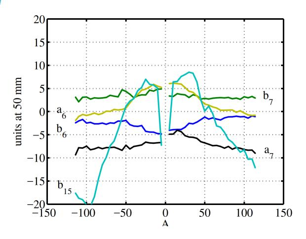
Multipoles measured at nominal current (105 A) and expressed in units at reference radius of 50 mm
