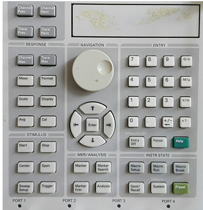
Figure 2. Button panel of the VNA.
