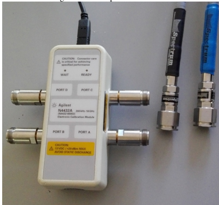
Figure 3. Electronic calibration device (left) and two probes of the VNA (right).
