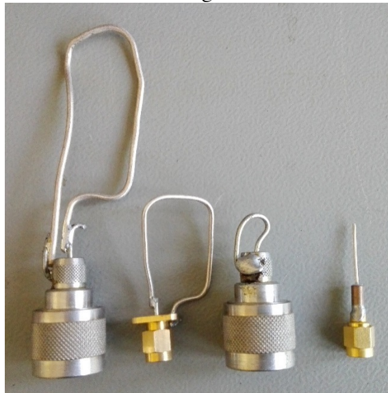
Figure 4. Different magnetic (three on the left) and electric probes.
