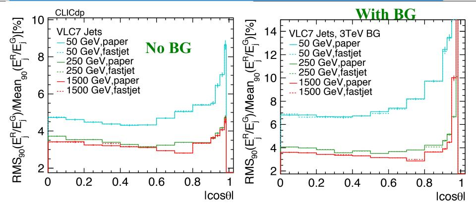
Compare the paper beam distance and the fastjet distance of VLC on one plot, solid: fastjet version, dashed: paper version
