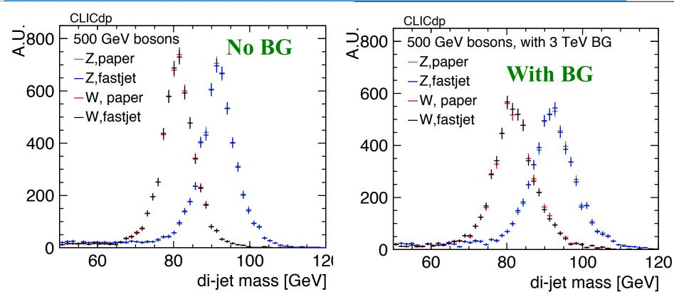
Compare the paper beam distance and the fastjet distance of VLC on one plot, checked for all bosons energies (same result for the other energies) →almost no differences, both beam distance measures lead to very similar results
