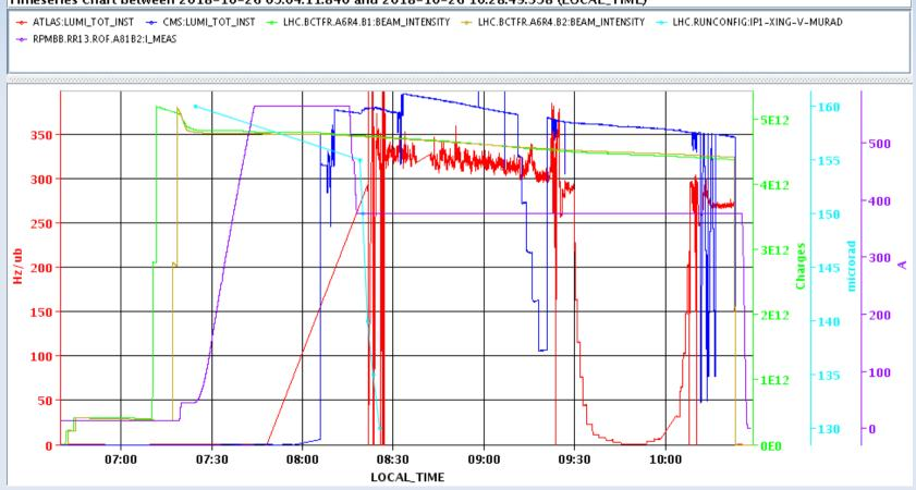
Pile-up about 130 (i.e. ~ HL-LHC design) were reached with 25ns beams
