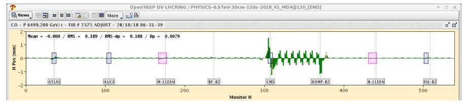
Measured bump of 2.3 sigma from IR6 to IP5
