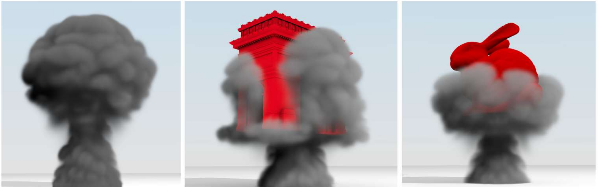
Fig. 1: Smoke simulation using our system - our method is capable of fast and accurate simulation of the Euler Equations for incompressible fluid flow at interactive frame-rates. Videos can be found at: http://cims.nyu.edu/~schlacht/CNNFluids.htm .
