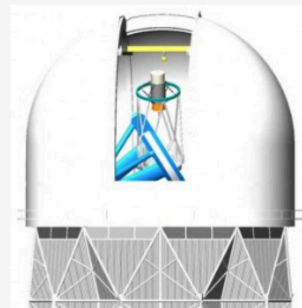
A model of the Mayall telescope with a DESI Prime Focus Assembly
