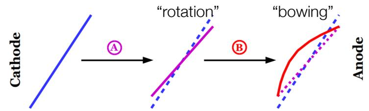
**Space Charge:** due to accumulation of slow-drifting ions from high rate of c.r. on surface, producing Drift Field distortion from nominal uniform E
