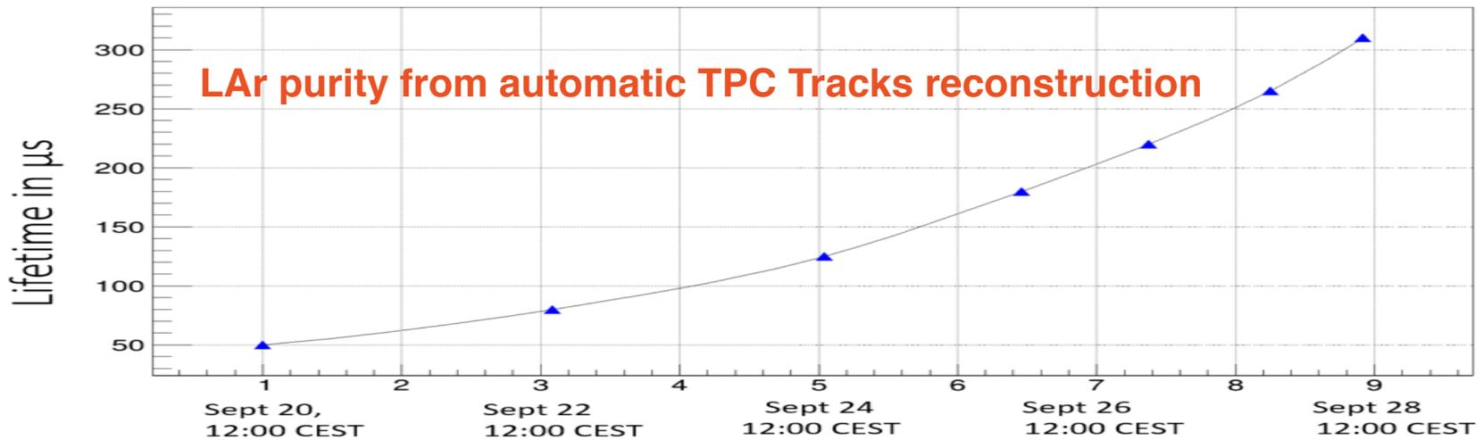
Initial low Purity, Recirculation ON, start noting Space Charge effects (ion accumulation)
