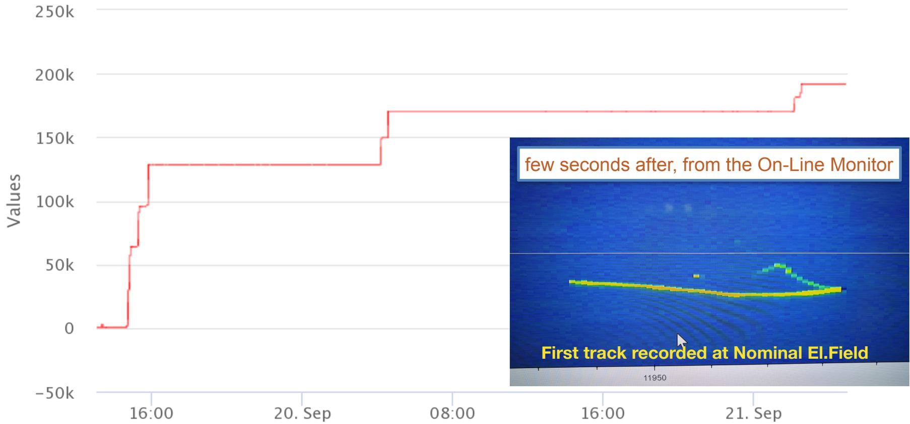
**HV Ramp from 0 to 180 kV (Nominal) successfully completed**
