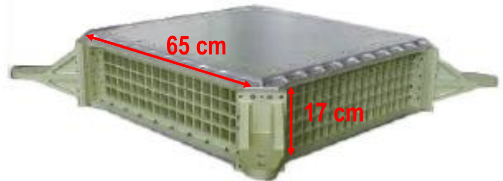
ECAL support structure
