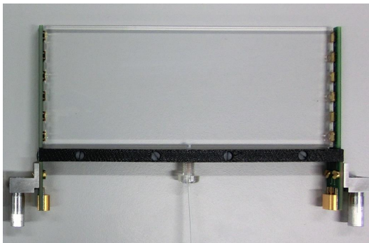
A scintillator counter readout with 6-series SiPM chain at both ends
