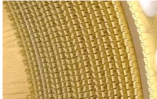
Highly granular drift cells formed by thin wires soldered on PCBs (no feedthrough & crimping)
