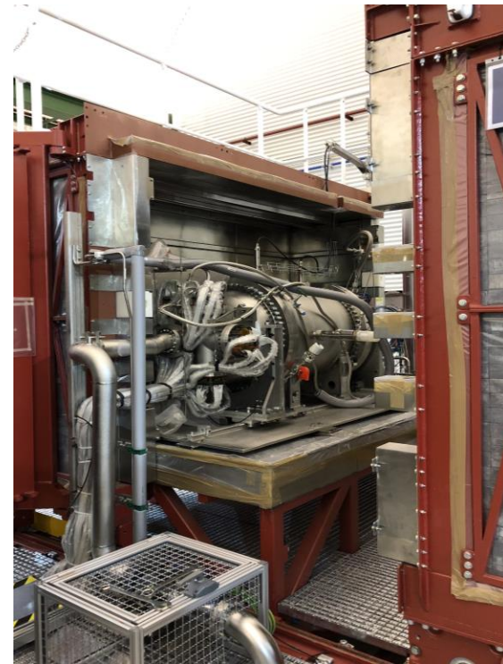
NEXT-NEW Vessel in its housing at Canfranc, Spain
