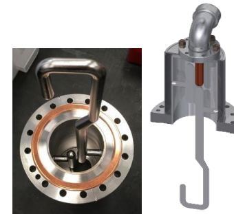
HHOM damper fabricated at JLab
