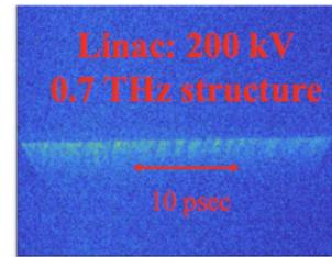
Time profiles showing the dependence of the time resolution on the linac voltage.
