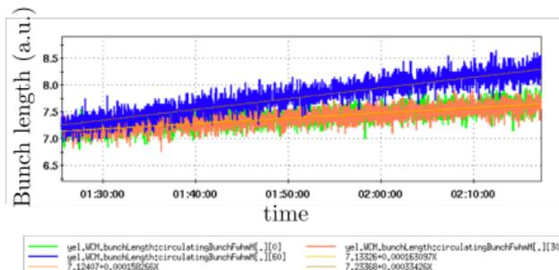
Heating of ion beam was occurring only with a perfect overlap of the beams and high FEL gain. Reducing the FEL gain eliminated the heating.
