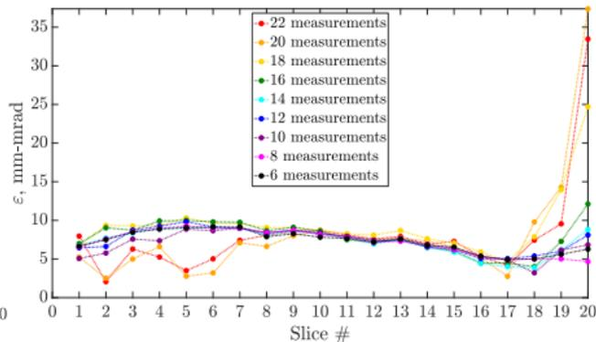
The slice emittance in the central part of the beam doesn't show any variations which could have led to a reduction of the ion imprint.
