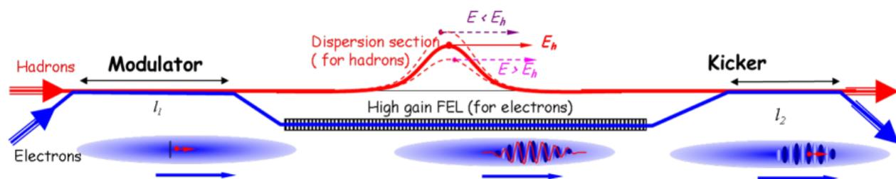
The electron and hadron beams co-propagate in a vacuum along a straight line in the modulator and kicker with the same velocity:
