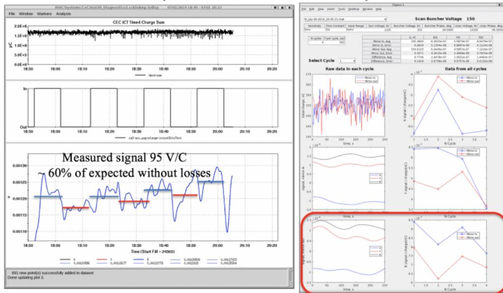
The base line was measured for modestly (4-fold) compressed beam with 1.5 and 0.3 nC charges per bunch in relaxed LEBT lattice. Averaged over 4 long scans the lock-in amplifier MDM signal was **105 V/C (24  $\mu$ W/A)** with **RMS error of 15 V/C (3  $\mu$ W/A)**. This value is at 40% level of synchrotron radiation that reaches the Cu mirror
