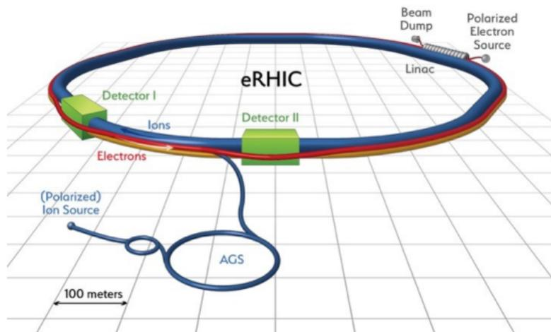
If CeC is successful and fully operational, eRHIC Linac/Ring configuration could reach  $2 \cdot 10^{33}$  luminosity with 5 mA polarized electron current.
