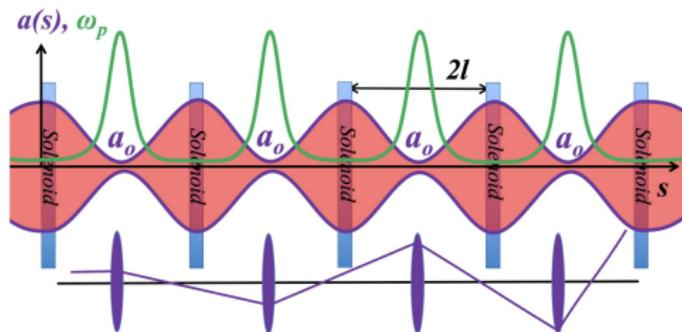
Propagating beam experiences density modulation with period of  $T = \frac{2l}{\gamma v}$ :
