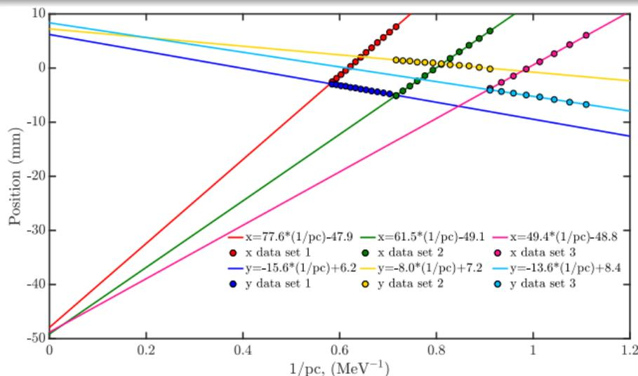
The y-intercept gives the direction of the gun axis for an infinitely rigid beam:
