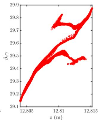
Longitudinal phase space at the exit of the 5-cell cavity.
