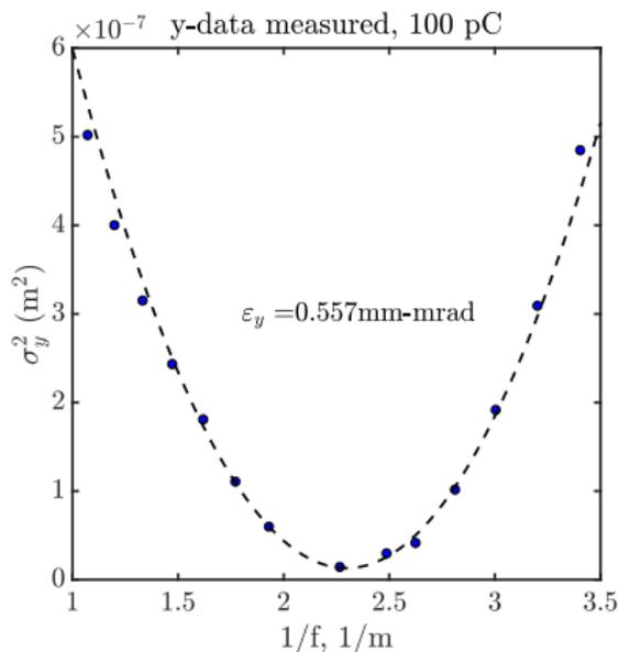
This data set was obtained for a 0.4 ns 100 pC electron beam at 1.25 MV gun voltage, and 1.34 mm diameter of the laser spot at the cathode.
