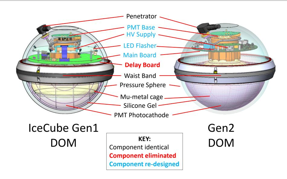
IceCube DOM with revised electronics: commercial 250 MSPS ADC and modern FPGAs for data buffering and compression
