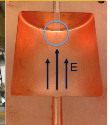
Qubit sensor + 10 GHz cavity mounted in new Fermilab mK test stand
