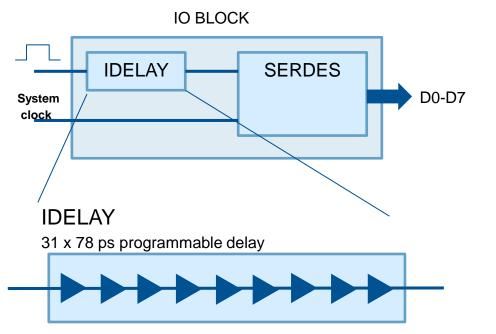
System clock maximum frequency 600 MHz
