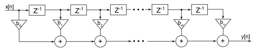
In one sampling cycle, we can make several multiplications, additions, subtractions filter cycles. It is possible to shorten the filter around 630/100~ 6 or 800/100~8
