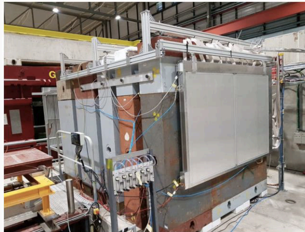
RPC prototypes built for muon flux and charm production
