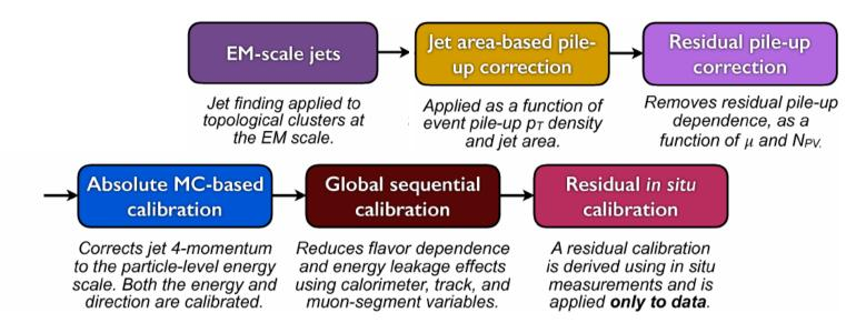
For large-R jets an additional grooming procedure (by default trimming, that removes  $k_{T} R = 0.2$  subjets with <5% of jet  $p_{T}$ ) can be applied before a dedicated MC and in-situ calibration
