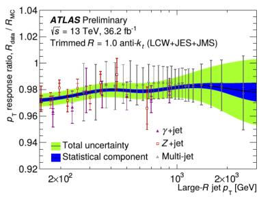
The results for the balancing methods are combined into a pt-dependent scale factor, used to rescale the whole jet 4-momentum.
