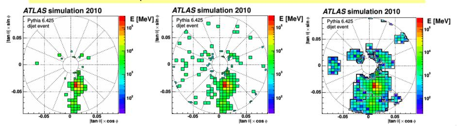
TopoClusters are then merged into jets using the anti-kt algorithm
