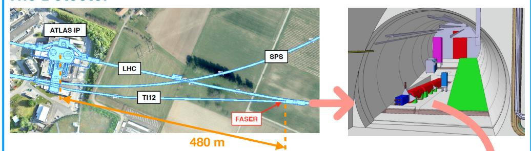
**Above:** The FASER detector will be positioned directly on the beam collision axis line-of-sight inside tunnel TI12, 480 m downstream from the ATLAS interaction point IP1 and a few meters from LHC beam line. The detector radius will be 10 cm, covering the millirad regime.
