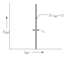
Figure 7-3. Ideal Constant Voltage Power Supply
