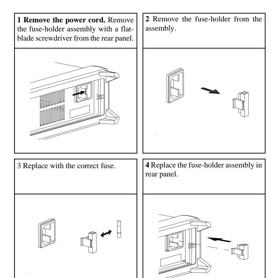
Verify that the correct line voltage is selected and the power-line fuse is good.
