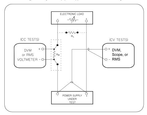
Figure A-1 Performance Verification Test Setup
