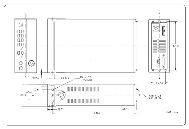
Figure 8-2. Dimensions for Rack mounting
