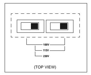
Figure 1-1. Line Voltage Selector (set for 115Vac)
