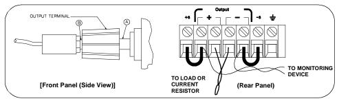
Figure A-2 Front/Rear Panel Terminal Connections
