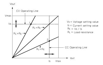
Figure 7-5. Output Characteristics
