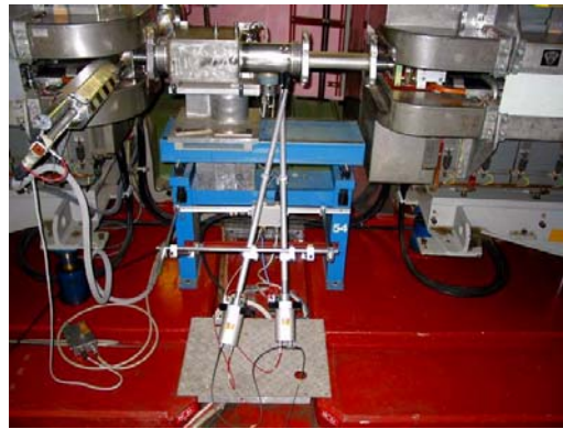
Figure 3-13: Fast wire scanner with scintillator and photomultiplier
