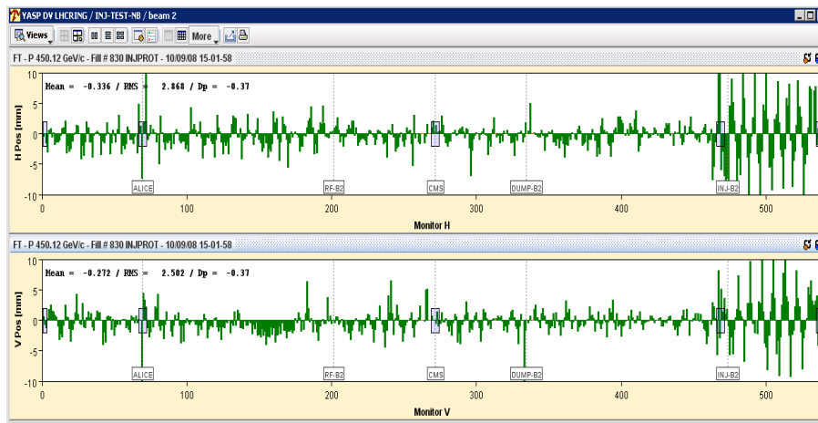
Figure 6-5: LHC trajectory measurement and orbit correction
