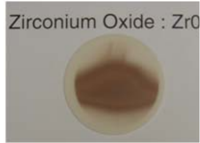
Figure 3-5: Alteration of the screen of exposure to ion beams
