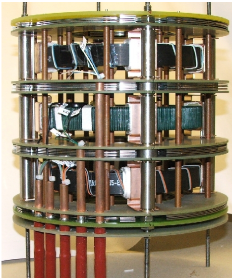
Figure 2-14: LHC DC current transformer
