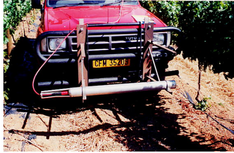
Fig.1 : MEDUSA detector mounted on a 4x4 vehicle during an in-situ mapping campaign.
