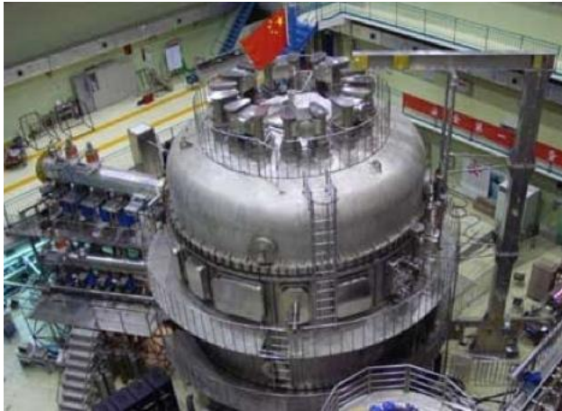
EAST: R = 1.7\text{m} , 2\text{MA} , 2006
