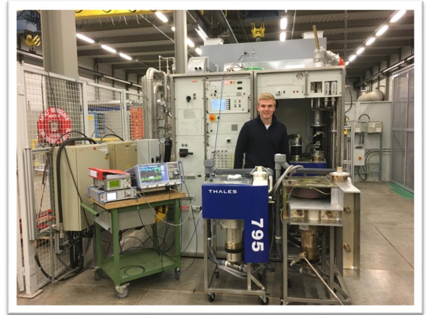
Left, Thales IOT Trolley operating at 800 MHz Right, modified by CERN trolley for an operation at 400 MHz James proudly showing the very good job done
